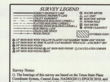
Coordinate System, Central Zone, NAD83(2011) EPOCH 2010, and boundary referenced to 1/2", 3/8" and 5/8" iron rods found and referred to the previous recorded plat.
